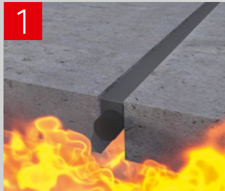
Joint de dilatation horizontal Sikasil®-670 Fire + Sika® Firestop profilé HD
